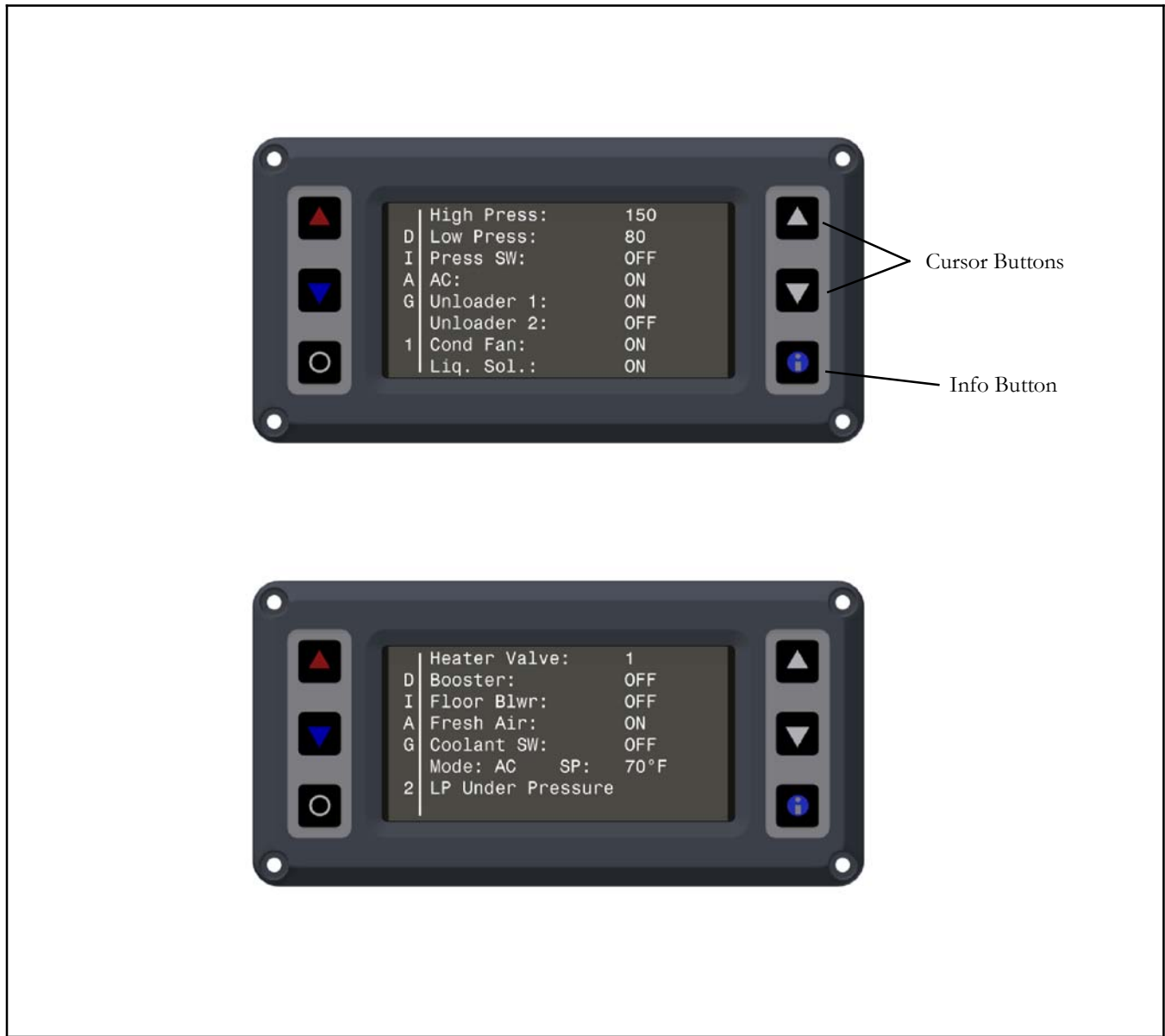
Figure 2-6 HVAC DIAGNOSTIC SCREENS
